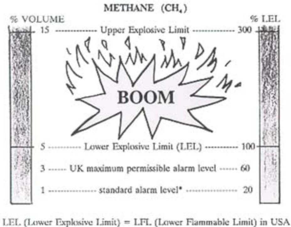
Figure 2. Upper and Lower Explosive Limits of Methane
